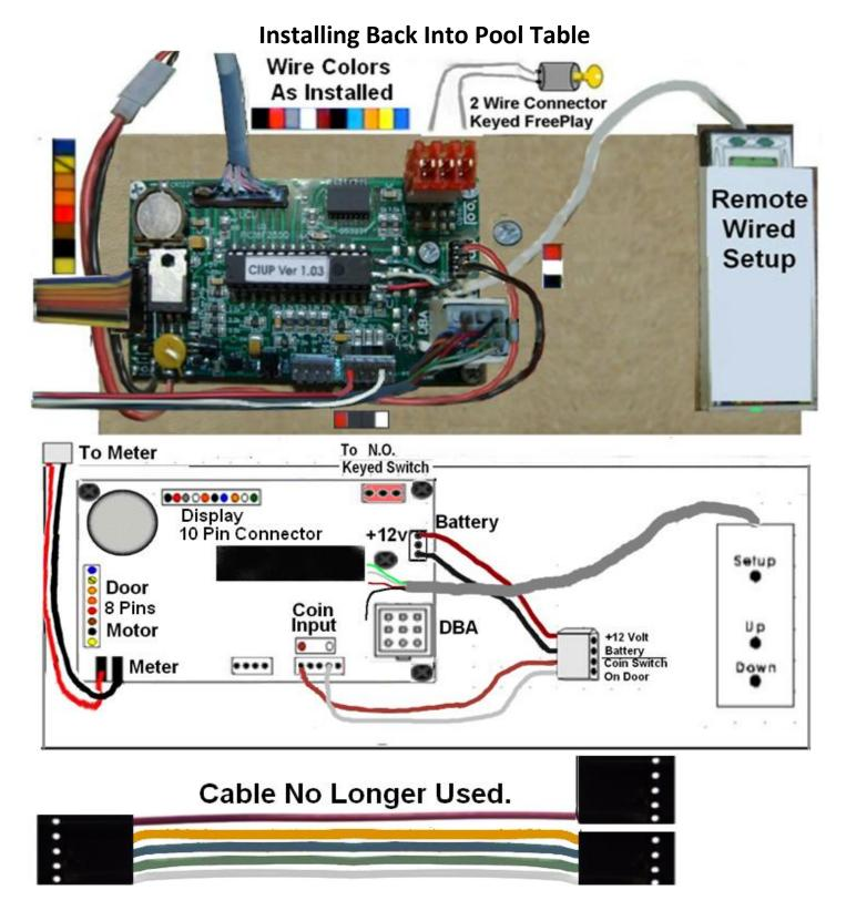
Keyed Switch Added for After Hours Free Play. Normally Open Circuit. Allows for use of table for free when Keyed Switch Closed Normal Operation unaffected, except if it has credits they will not be removed. Any Credits added during this time will work after Key Switched to Off. Reinstall In Original Location. See Top for Cable Reconnections. Factory Set at \$1.00 Per/Play, Bonus at \$5 and \$10 Next Setup Instructions:
