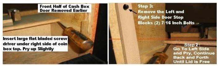
Remove and Save Cashbox Cover Cut off nails remaining in wood: Remove Door Wood Stop Blocks and Above Door.
