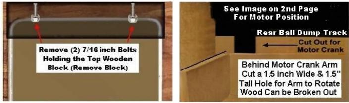
Using a Saw, Cutout an Area on Rear Ball Dump Track About ½ inch Right, of Left Cash Box Ledge About 1.5 X 1.5 inch.
