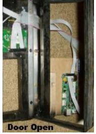
Return to the Left Side and Loosen the Center Hinge Screw . <u>Insert Left Spacer or Shim as needed to Secure the Assy,</u> Tighten the Center Hinge Screw Just Enoungh to Keep The Assy Solid. Now Remove one at a Time Top and Bottom Hinge Screws Replaceing them with 1 & ½ Wood Screw. Goto <u>Top Side Add Spacer & Shim</u> and Install (2)Wood Screws
